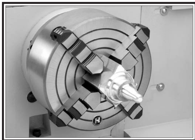
Figure 37. Example photo of non-cylindrical workpiece correctly mounted on the 4-jaw chuck.
